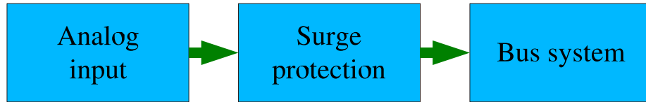
Figure 3.24: Analog Input Board block diagram.
